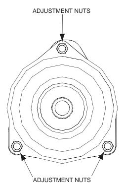
Figure 6-5. Clutch Air Gap Adjustment
